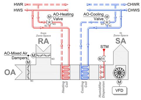
Schematic Description of Typical Air Handling Unit
